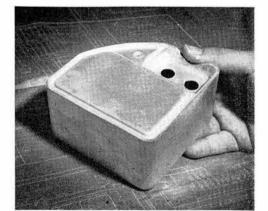
UNIQUE CAPABILITY of the electron beam welder in the Welding Laboratory is evident in the weld on this electronic component container. Most electron beam machines will weld only straight lines or circles, but the Sandia unit will weld any contour of a single plane. Roman Heuer (7512) drew up the specifications for the unit, the only one of its kind.
